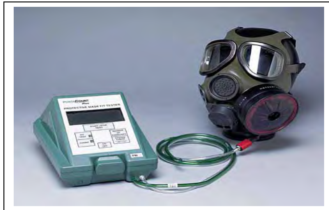
Figure A-6. M41 Protection Assessment Test System
